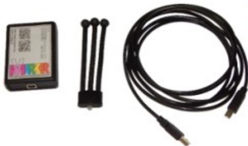
The *Vmarker IR-sensor USB™* is connected to the USB-port of the computer. The computer will recognize the sensor as a normal HID-device (a mouse). Together with an IR-pen (not included) you can make an interactive Whiteboard with your computer and beamer. You can easily make the IR-pen yourself, the IR-sensor is compatible with IR-pens used with the wii-mote, or when you also want extra functionality, you can purchase the special *Vmarker IR-pen Touch™*.
